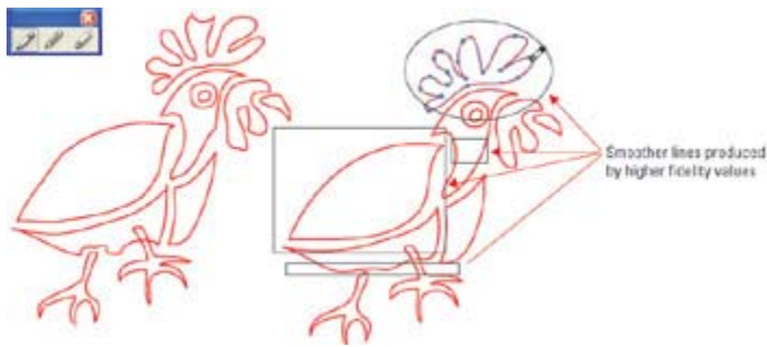
Figure 4-4: The drawing on the left, produced with a low fidelity value, is more jagged than the one on the right, produced with a higher value.
